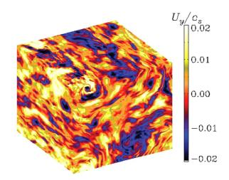
FIG. 2. Axial flow component  $U^{y}$  on the periphery of the domain for Run B2 with  $k_{\rm f}/k_1 = 5$  and Re = 460.
