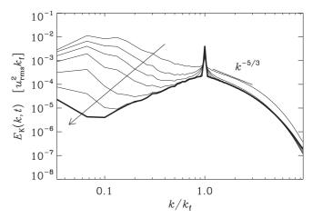
FIG. 9. Same as Fig. 8, but for Run C3 with a finite amplitude initial condition, giving Re = 100, at  $t/\tau$  = 20, 100, 200, 500, 1000, and 1700. Here  $k_f/k_1$  = 30, Co = 0.5, and 576<sup>3</sup> mesh points.
