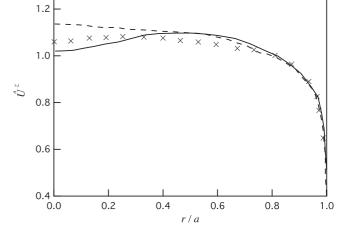
FIG. 11. Mean axial velocity profile in the turbulent swirling flow. The normalized mean axial velocity  $\hat{U}^z (= U^z/U_m, U_m$ : bulk velocity defined by  $U_m = \int_0^a U^2 2\pi r \, dr/\pi a^2)$  is plotted against the scaled radius r/a (*a*: pipe radius): ×, experiment; —,  $K - \epsilon - H$  model; --, standard  $K - \epsilon$  model. Redrawn from Ref. [6].
