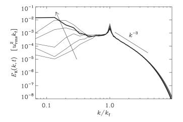
FIG. 6. Inverse transfer seen in kinetic energy spectra at  $t/\tau = 100$ , 200, 500, 1000, 2000, and 3500, for Run A with  $k_f/k_1 = 15$ , Re = 60, Co = 0.7, and 288<sup>3</sup> mesh points. The arrow denotes the temporal evolution. The bold line indicates the last time in the plot.
