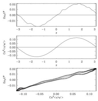
FIG. 5. Mean axial velocity  $U^{y}$  (top), turbulent helicity multiplied by rotation  $C_{0}^{2} \langle \mathbf{u}' \cdot \boldsymbol{\omega}' \rangle = (2\omega_{\rm F}\tau)^{2}H$  (middle), and their correlation (bottom) for Run A with  $k_{\rm f}/k_{\rm I} = 15$  and Re = 60 at the developed equilibrium stage (averaged over time from  $t/\tau = 0$  to 2000).
