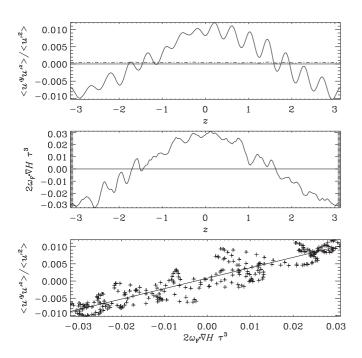
FIG. 4. Reynolds stress  $\langle u'^y u'^z \rangle$  (top), helicity-effect term  $(\nabla H)^z 2\omega_F^y$  (middle), and their correlation (bottom) for Run A with  $k_f/k_1 = 15$  and Re = 60 at the early stage of development (averaged over time from  $t/\tau = 40$  to 200).
