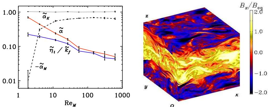
Figure 1: Dependence of  $\alpha$  effect and turbulent magnetic diffusivity,  $\eta_t$ , on the magnetic Reynolds numbers, as obtained by the test-field method in the nonlinear regime (left) for large-scale magnetic fields of equipartition strength (right) [4].
