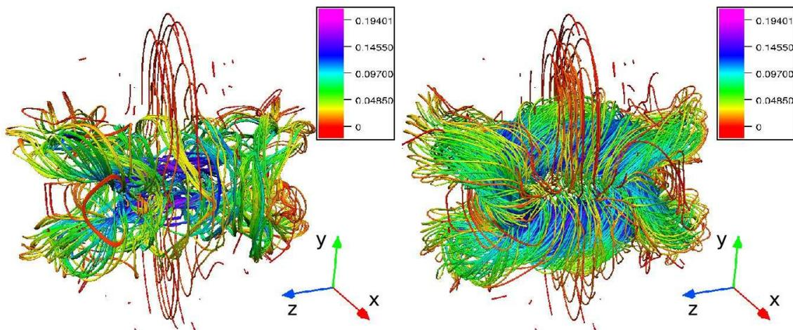
Figure 2: Magnetic field configurations of decaying triply-interlocked flux rings with zero helicity (left) and finite helicity (right). The configurations on the right decays much more slowly, because magnetic helicity conservation controls the decay rather than the qualitative degree to which the rings are interlocked [9].
