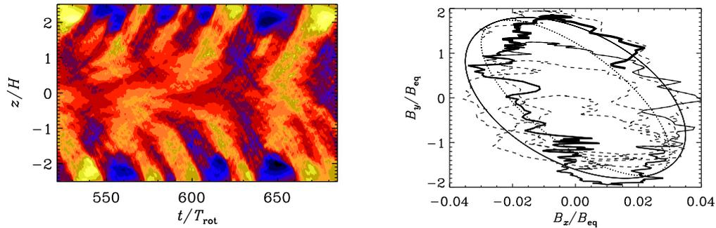
Figure 4: Space-time diagram of the  $\overline{B}_y$  component of the mean magnetic field driven by the magneto-rotational instability (left). Note the  $3\pi/4$  phase shift between  $\overline{B}_x$  and  $\overline{B}_y$  (right) [14].
