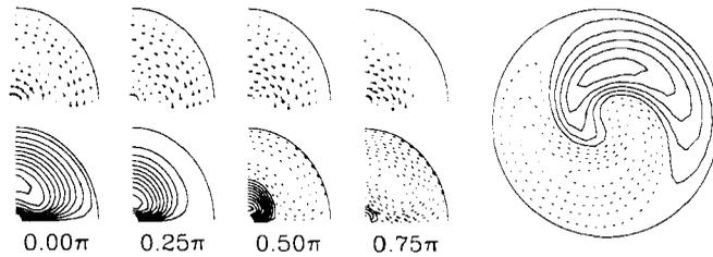
**Figure 3** Field configuration for the first A1 mode. On the right are shown level contours of the vertical field component in the disc plane. The radial and azimuthal fields are zero in the plane. Otherwise the same as Figure 2.
