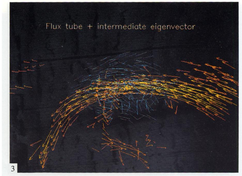
Fig. 3. Flux tube (from red to yellow as field increases) together with the eigenvector  $e_1$  (blue), corresponding to the direction of compression, in a ball with a radius of 4 mesh points around the point of maximum magnetic field strength.
