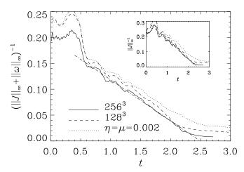
FIG. 3. Evolution of  $1/\|\mathbf{J}\|_{\infty}$  and  $1/(\|\mathbf{J}\|_{\infty} + \|\boldsymbol{\omega}\|_{\infty})$ . r = 0.5 for  $\beta_0 = 2$ . Solid and dashed lines refer to ideal calculations with different resolution and the dotted line is for a resistive calculation with  $\eta = \mu = 0.002$ . The dash-dotted line gives a linear fit to the data. Inset is  $1/\|\mathbf{J}\|_{\infty}$ .
