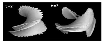
FIG. 2. Three-dimensional level surfaces of the magnitude of the current density in the resistive calculation. t=2 shows a double saddle surface, which at t=3 is broken up into two disjoint pieces.
