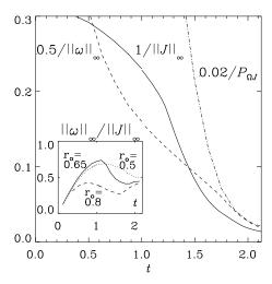
FIG. 4. Comparison of the evolution of  $1/\|\mathbf{J}\|_{\infty}$ ,  $1/\|\boldsymbol{\omega}\|_{\infty}$ , and  $P_{\Omega J}$  for  $r_0=0.65$ . The inset shows  $\|\boldsymbol{\omega}\|_{\infty}/\|\mathbf{J}\|_{\infty}$  for r=0.5, 0.65, and 0.8, all of which are converging to  $\|\boldsymbol{\omega}\|_{\infty}/\|\mathbf{J}\|_{\infty} \approx 0.5$ , demonstrating possible self-similarity.
