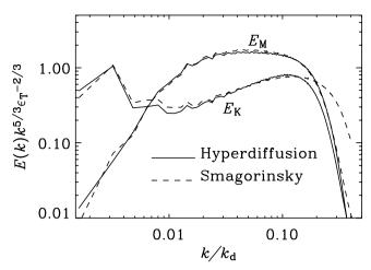
**Fig. 5.** Magnetic and kinetic energy spectra for runs with  $512^3$  mesh points and hyperviscosity and hyper-resistivity (solid line) and Smagorinsky viscosity and hyper-resistivity (dashed line). Note the mutual approach of kinetic and magnetic energy spectra before entering the dissipative subrange.
