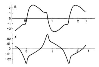
**Fig. 12.** Evolution of toroidal and poloidal fields, B and A, respectively, from the paper by Stix (1972). Note the similarity in the evolution of his model and that in the direct simulation shown in Fig. 10, with a more spiky behavior of the poloidal field compared to the toroidal field. [Adapted from Stix (1972).]
