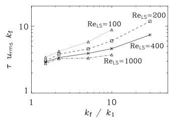
**Fig. 9.** Strouhal number as a function of  $k_{\rm f}/k_{\rm 1}$  for different values of Re<sub>LS</sub>, i.e. the large scale Reynolds number. The resolution varies between  $64^3$  meshpoints (Re<sub>LS</sub> = 100) and  $512^3$  meshpoints (Re<sub>LS</sub> = 1000).
