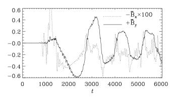
**Fig. 10.** Evolution of  $\overline{B}_x$  and  $\overline{B}_y$  at  $x = -\pi$  and z = 0. Note that  $\overline{B}_x$  has been scaled by a factor -100. [Adapted from Brandenburg et al. (2001).]
