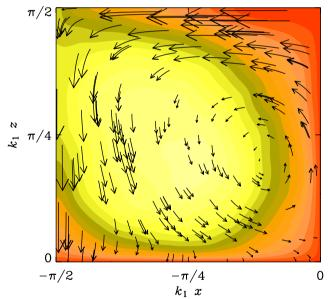
**Fig. 19.** (online colour at www.an-journal.org) Same as Fig. 17, but for  $\alpha < 0$ , so the turbulence is forced with positive helicity. Note the anti-clockwise sense of the poloidal field, corresponding to negative magnetic helicity, consistent with  $\alpha < 0$ .
