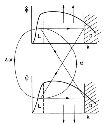
**Fig. 1.** A sketch from the original review by Stix (1974) where he illustrates the role of a turbulent cascade in converting large scale poloidal and toroidal flux into small scale fields where it can be converted into heat by microscopic resistivity.
