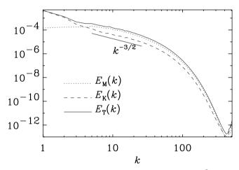
**Fig. 3.** Magnetic, kinetic and total energy spectra.  $1024^3$  meshpoints. The Reynolds number is  $u_{\rm rms}/(\nu k_{\rm f})\approx 960$ . [Adapted from Haugen et al. (2003).]
