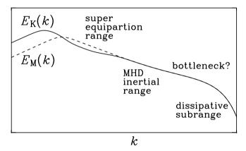
**Fig. 6.** Sketch of the anticipated kinetic and magnetic energy spectra in the large Reynolds number limit for  $\Pr_M=1$ . Note the slight super-equipartition just to the right of the peak of  $E_{\rm M}(k)$  and the asymptotic equipartition for large wavenumbers.
