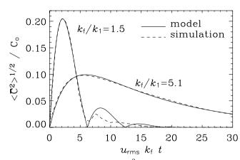
**Fig. 8.** Passive scalar amplitude,  $\langle \overline{C}^2 \rangle^{1/2}$ , versus time (normalized by  $u_{\rm rms}k_{\rm f}$ ) for two different values of  $k_{\rm f}/k_{\rm l}$ . The simulations have  $256^3$  meshpoints. The results are compared with solutions to the non-Fickian diffusion model. [Adapted from Brandenburg et al. (2004).]
