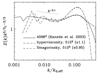
**Fig. 4.** Comparison of energy spectra of the  $4096^3$  mesh points run of Kaneda et al. (solid line) and  $512^3$  mesh points runs with hyperviscosity (dash-dotted line) and Smagorinsky viscosity (dashed line).
