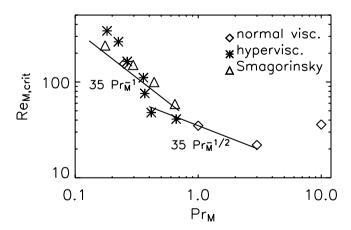
**Fig. 7.** Dependence of the critical magnetic Reynolds numbers as a function of the magnetic Prandtl number using for the direct simulations (Haugen et al. 2004), indicated by diamonds, compared with results using hyperviscosity (asterisks) or Smagorinsky viscosity (triangles).
