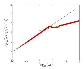
FIG. 4. (Color online) Mean energy of the particles as a function of time for run R2; see Table I. The two straight lines are fits (in the least-squares sense) with slopes 1.95 and 0.77 for small t and large t, respectively.
