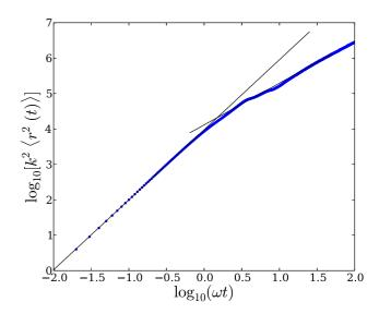
FIG. 1. (Color online) Average displacement  $\langle r^2 \rangle$  as a function of time for particles in a stationary ABC magnetic field ( $\omega=0$ ). The ordinate is normalized with  $k^2$ . The two straight lines to the left and right of the curve are fits with slopes 1.9 and 1.1, respectively.
