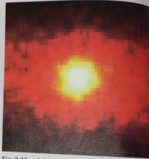
Fig. 2-10. A Neutrino Image of the Sun. This view of the Sun is from the Super-Kamiokande (Super-K) experiment in Japan. Brighter colors represent a larger flux of neutrinos. Three hundred days of data were collected to produce this neutrino image of the Sun. The picture covers a significant fraction of the sky; however most of the neutrinos are coming from the vicinity of the solar core. (Courtesy of NASA and Robert Svoboda at Louisiana State University)
